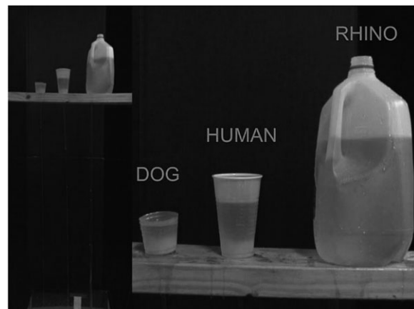
Figure 5 Image from a video illustrating the relatively constant duration of animal urination regardless of the animal size. The containers on the right contain the bladder volumes of a rhino, human and dog. Long pipes representing urethras of the appropriate dimension are installed beneath the bladder. These pipes enable the containers of vastly varying volume to empty in the same duration
